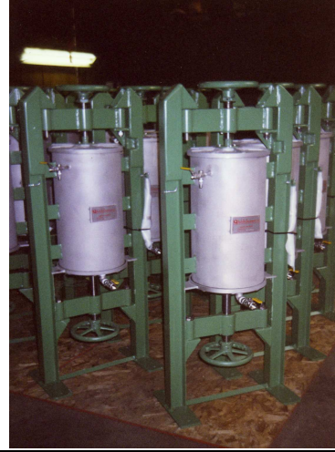
12 ea. QPEC 12" 316 ss Pressure Filters
