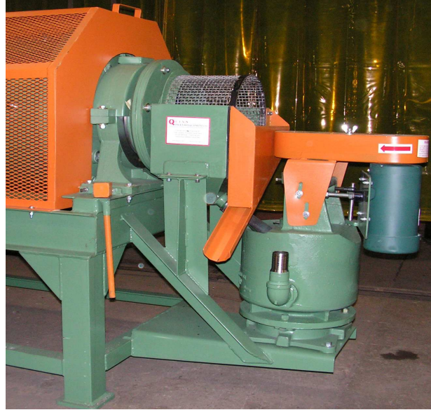
QPEC 1" Vertical Sand Pump mounted to 24" x 64" Ball/Rod Mill
