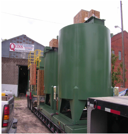
2 ea QPEC 8' x 10' Thickener Tanks skid mounted with Hopper-Belt Feeder being shipped to Australia
