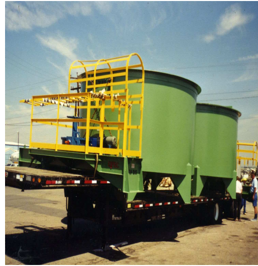
2 ea QPEC 14' x 8' Thickener Tanks in transit
